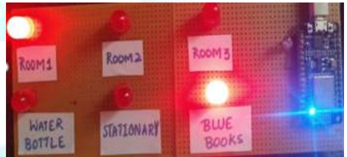
Fig. 7 Wi-Fi module interface with the LED keypad
